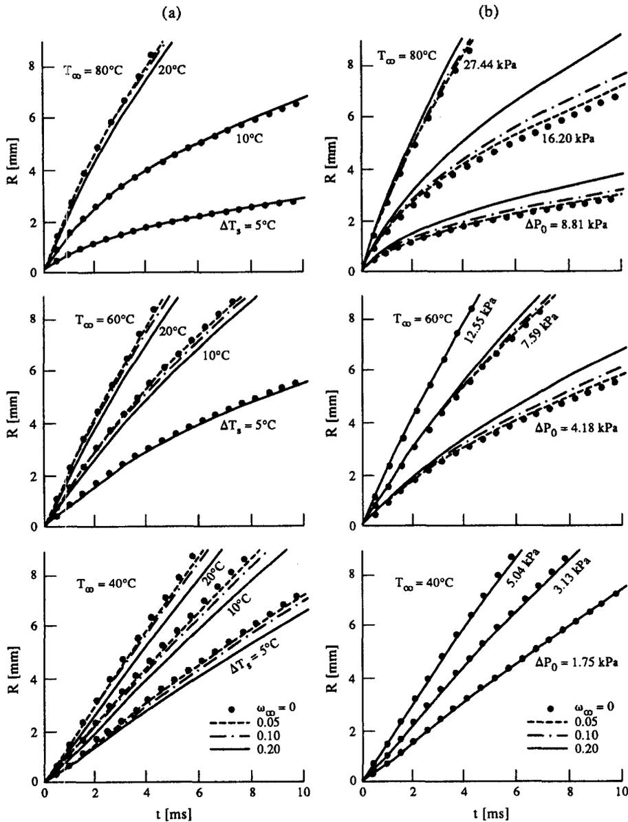
Fig. 2. The bubble growth histories in aqueous NaCl solutions at four solute mass fractions ( $\omega_\infty$ ), at three given solution temperatures ( $T_\infty$ ), from ref. [20], for three fixed values of (a) the superheat ( $\Delta T_s$ ); (b) the initial pressure difference ( $\Delta P_0$ ).
