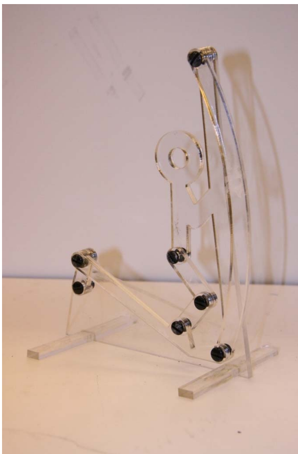
Figure 4: Photograph of an elliptical machine prototype. Note that the main frame serves as a main stand and the body of the person is rigidly attached to this stand.
