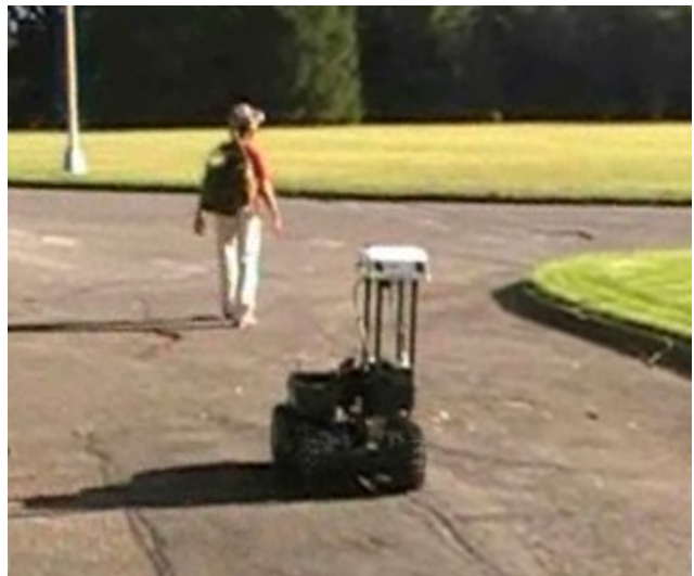
Figure 1. Our system in action during a leader-follower experiment. The robot, equipped with stereo cameras and an IMU, is autonomously following an operator wearing the same sensors on his helmet. The system uses visual navigation with robot-to-helmet landmark matching capability to achieve non-line-of-sight, tag-along robot capability. The operator can move freely in the environment, walking, running, looking around and walking backwards.
