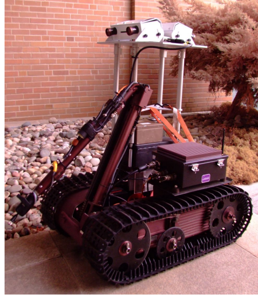
Figure 3. The VideoTrek follower system installed on a mobile robot. The sensors are in the white boxes on the platform and the processor is in a black box visible on the side of the robot.
