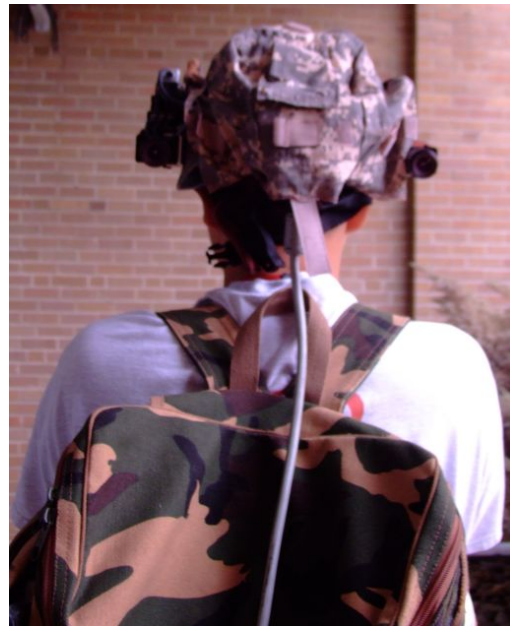
Figure 4. The VideoTrek leader system. The cameras are visible on the sides of the helmet. The gray cable connects the sensors on the helmet with the processing inside the backpack.
