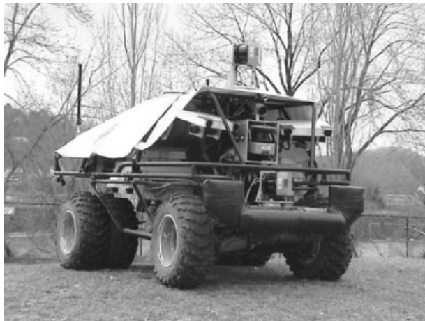
Figure 4. A picture of the autonomous ground vehicle. Note the two stereo heads mounted in the front. For this platform, a specifically tailored version of the camera motion estimation system is used. The available stereo input is leveraged to obtain even more stable visual odometry. The feature tracking front end is essentially the same, but the known stereo geometry is used in the robust motion estimation. The somewhat more difficult relative orientation step used in the single camera case can thus be avoided. The system then essentially performs triangulation of scene points followed by estimation of pose from the structure that was previously determined. A significant advantage is that in this mode, the system can perform well despite little or even no camera motion.
