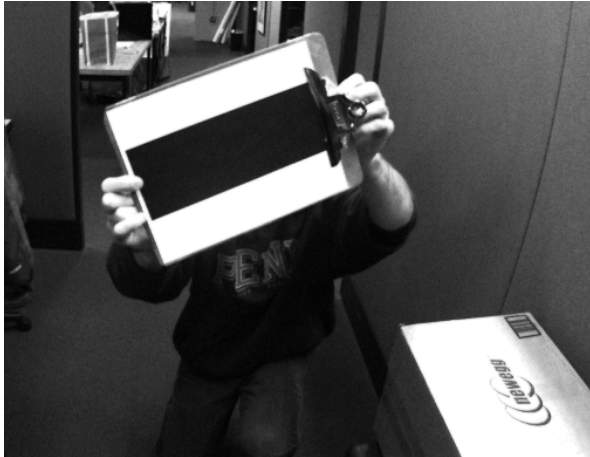
Fig. 2. A single camera frame from the calibration data set showing the calibration object. The object consists of a black line on a white sheet of paper. We detect the white-to-black transition looking from the top of the image.
