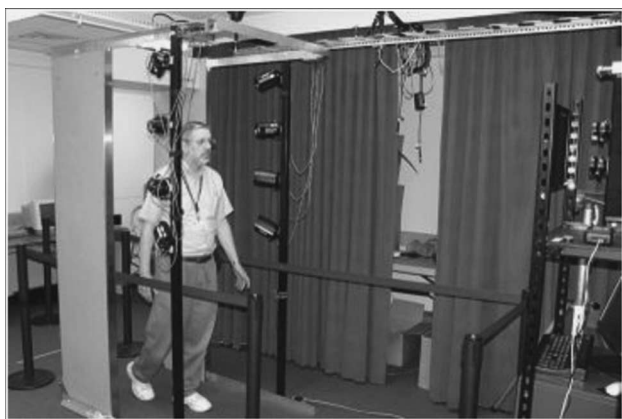
Fig. 6. Illustration of the concept of operation for the IOM system. The panels behind the subject are the sides of a commercial metal detector. The stanchions just in front of the subject support an array of NIR illuminators. The camera package is at the far right of the subject.
