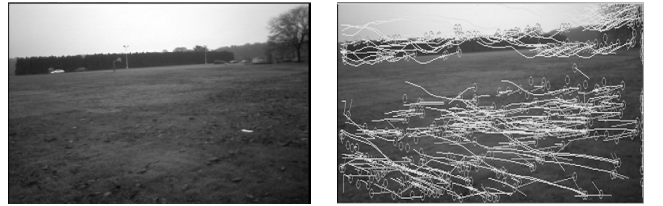
Figure 2: Input frame (left) and feature tracker output (right). Circles represent current feature locations and curves are feature tracks through the image.
