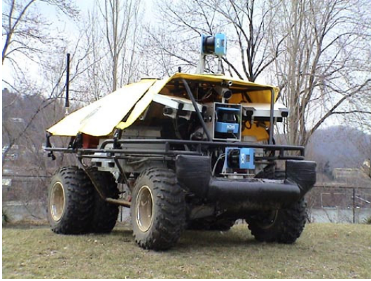
Figure 4: A picture of the autonomous ground vehicle. Note the two stereo heads mounted in the front. For this platform, a specifically tailored version of the camera motion estimation system is used. The available stereo input is leveraged to obtain even more stable visual odometry. The feature tracking front end is essentially the same, but the the known stereo geometry is used in the robust motion estimation. The somewhat more difficult relative orientation step used in the single camera case can thus be avoided. The system then essentially performs triangulation of scene points followed by estimation of pose from the structure that was previously determined. A significant advantage is that in this mode the system can perform well despite little or even no camera motion.
