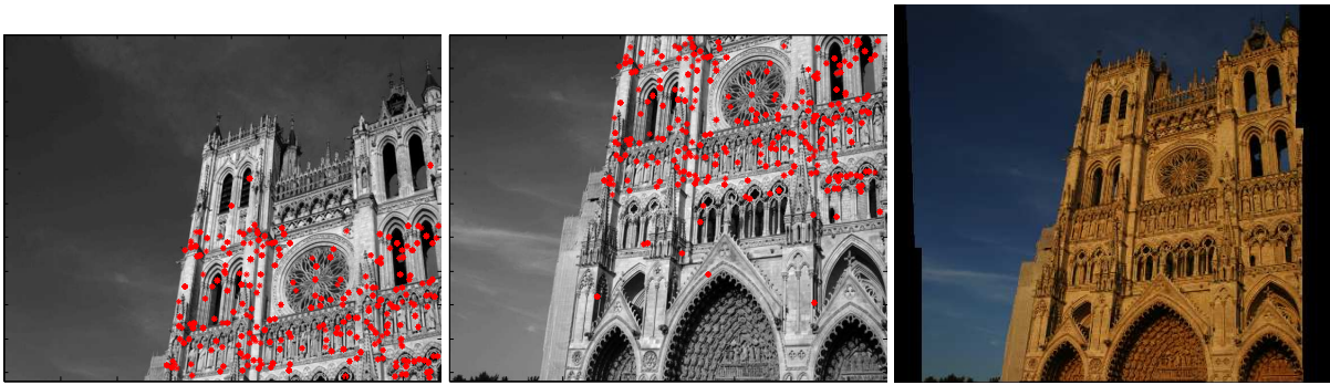
Figure 8. The matched SIFT features on high quality images and the resulting panorama generated with single precision arithmetic using the reduced template and RANSAC.
