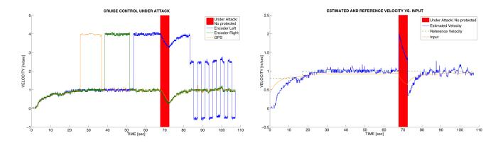
Figure 6: Experimental results; (a) Comparison of velocity estimated from the encoders' and GPS measurements; (b) Reference speed, the estimated speed, and the input applied to the motors.
