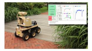
Figure 5: Deployment of the LandShark on a tiled pathway. The picture in the picture displays the user interface used in experiments.
