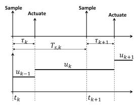
Figure 1: Scheduling sampling and actuation.
