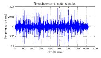
Figure 7: Times between consecutive left encoder measurements.
