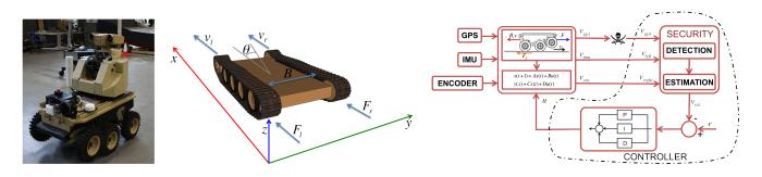
Figure 4: LandShark unmanned ground vehicle; (a) The vehicle; (b) Coordinate system and variables used to derive the model; (c) Control system diagram used for cruise control.
