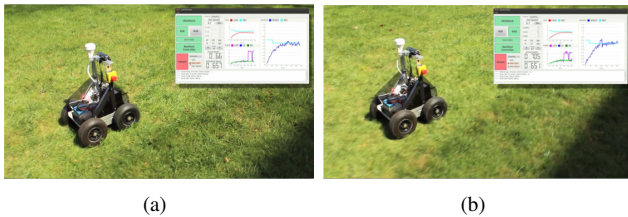
Fig. 9. Snapshots of the deployment of the MiniShark UGV on a grass field inside the University of Pennsylvania. The robot is in cruise control and one by one each sensor is compromised with a constant attack. Figure (a) shows the implementation of the RSE, while (b) depicts the RAE strategy.
