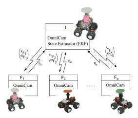
Fig. 2. Communication network architecture. All computation is carried out on the leader who receives the measurements (the angle  $\eta_i$ ) from all the follower and transmits the control input  $(v_{F_i}, \omega_{F_i})^T$ .
