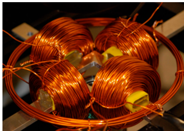
Fig. 1. Five electromagnetic coils, four in-plane and one out-of-plane, are mounted on an optical microscope to actuate the microtransporters.
