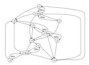
Fig. 2: Automaton for the Hide and Seek example
