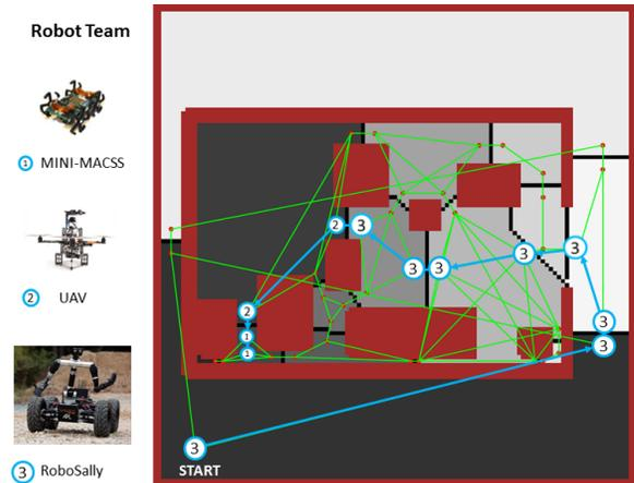
Fig. 1. Depiction of two-dimensional planning for the nested marsupial system described in [8, 6], consisting of a carrier UGV (3), a quadcopter UAV (2), and a miniature UGV (1). Red represents occupied space, grayscale represents the catchment basin, green represents the multi-graph, and black the watersheds.
