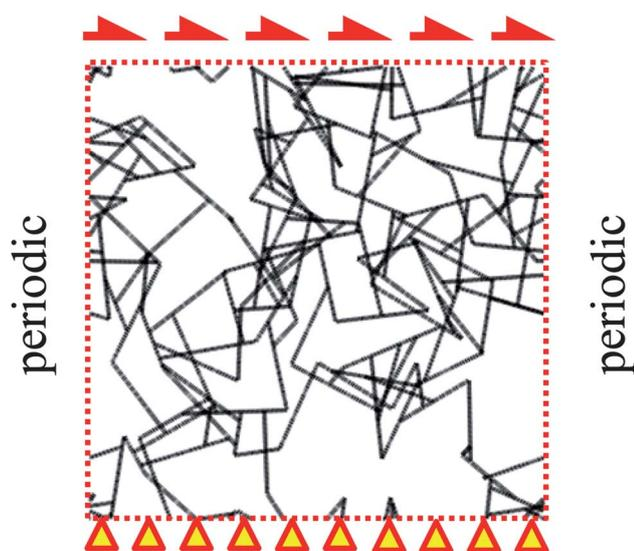
**Fig. 1** Initial configuration of a typical network. Dangling ends are removed and the boundary of the computational window (red dashed lines) along with the kinematic boundary conditions (b.c.'s) are shown.
