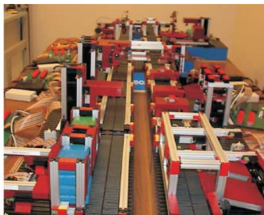
Fig 1. (a) Example of a mini-factory layout with a U-shaped conveyor belt across all operation units. (b) A FireFly wireless sensor node with a microcontroller and radio
