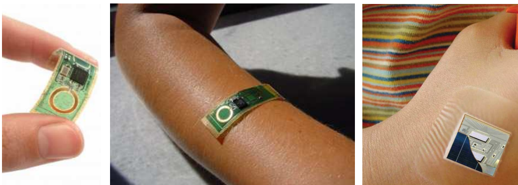
Fig 4. Models of the proposed on-body smart health-strip for contextual electrocardiogram monitoring. The health-strip will feature a multi-channel ECG sensor, accelerometer, microSD slot and wireless radio.
