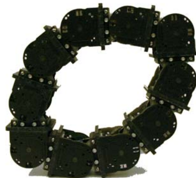
Figure 2: Rolling wheel configuration for a modular robot.
