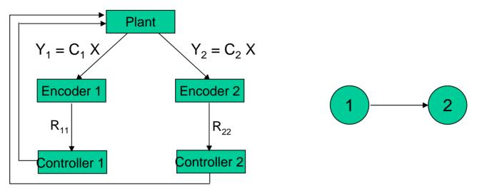
• Assume:  $C_1 (zI - A)^{-1} B_2 = 0$ . The actions of controller 2 are not observed by controller 1.  $A + B_1 K_1 C_1 + B_2 K_2 C_2$  is stable.
