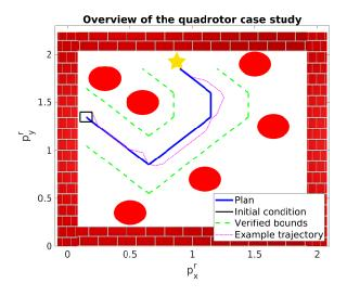
Figure 5: Overview of the quadrotor case study, as projected to the (x, y)-plane. The quadrotor's goal is to follow its planner in order to reach the goal at the top (star) without colliding into obstacles (red circles). We have verified that, starting from any state within the shown set of initial conditions, the quadrotor will not deviate from its plan by more than 0.32m (and hence will not collide into any obstacles).
