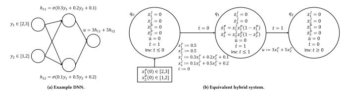
Figure 2: Small example illustrating the transformation from a DNN to a hybrid system.
