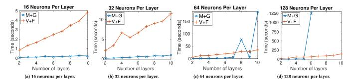
Figure 6: Comparison between the verification times of Verisig+Flow\* (V+F) and the MILP-based approach with Gurobi (M+G) for DNNs of increasing size. In each figure, the number of neurons is fixed and number of layers varies from two to 10.
