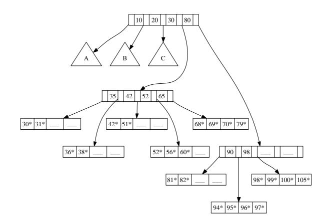
3. Name a search key value such that inserting it into the original tree would cause an increase in the height of the tree.
