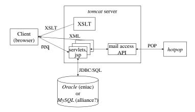
Figure 1: Basic system architecture
