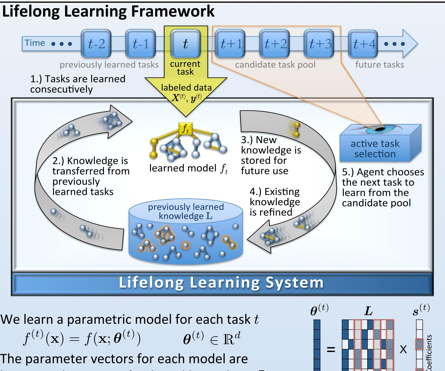
We learn a parametric model for each task tThe parameter vectors for each model are linear combinations of a shared latent basis L  $\boldsymbol{\theta}^{(t)} = \mathbf{L} \boldsymbol{s}^{(t)} \quad \mathbf{L} \in \mathbb{R}^{d imes k}, \ \boldsymbol{s}^{(t)} \in \mathbb{R}^{k}$
