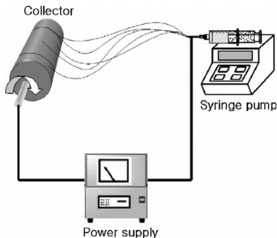
Figure 2a: Basic schematic diagram of electrospinning..
