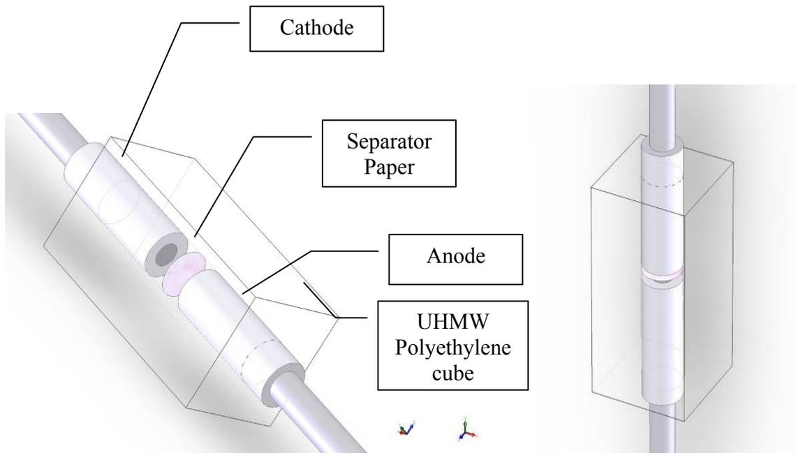
**Figure 3.** Prototype setup for a supercapacitor device.
