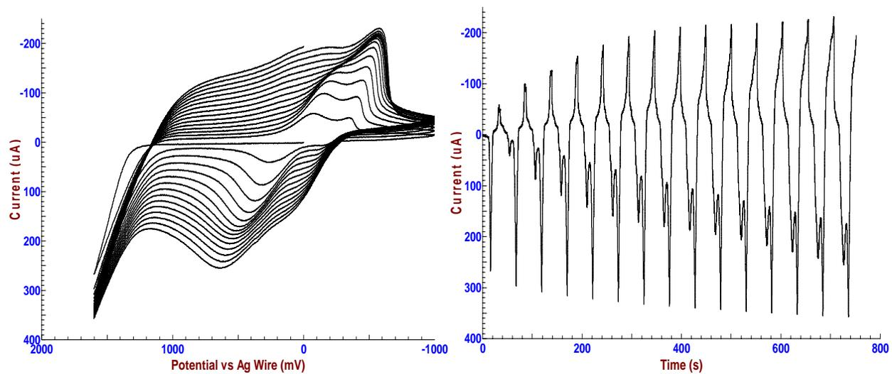
**Figure 4.** Cyclic voltammogram over 30 sweeps of ProDOT in EMI-BTI/TEA-BTI/PC at 100 mV/s (a) and corresponding current vs time trace (b).
