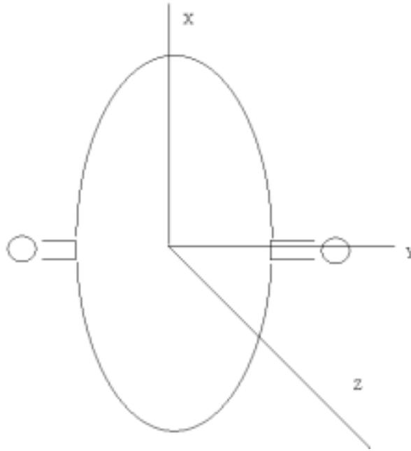
Pitch is defined as rotation around the Y-axis, and yaw is rotation about the Z-axis. Roll, which is rotation about the X-axis, is negated.
