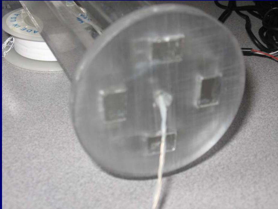
There was significant frictional error between the cable and the top of the Tower. Attempts to reduce the error did not work as well as hoped.
