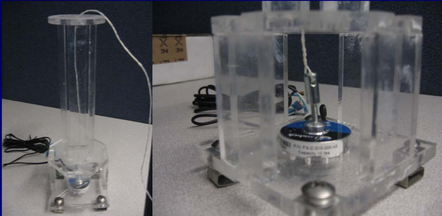
Towers have cables attached to the iLoad Mini Load Sensors, using screws with holes. They are also built to align and read the cable tension.
