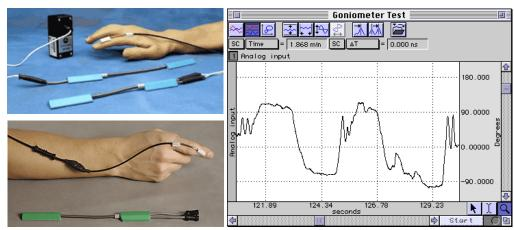
In the example above, the TSD130A was connected directly to a DA100C amplifier, the DA100C gain was set to 1,000, and AcqKnowledge was used to calibrate the signal to provide angular measurements from approximately +90° to -90°.
