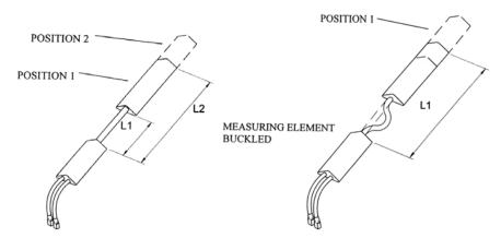
If a light force is now applied, pushing the two endblocks linearly towards each other, the only way the distance L1 can decrease in length is if the measuring element buckles.
