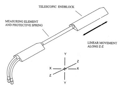
Assuming the goniometer is mounted correctly (as outlined here), the outputs of the two channels are independent of linear displacements along axis Z-Z.
