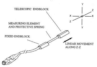
The goniometer does not measure rotations about axis Z-Z, though this movement is permitted without reduced life or damage occurring. This goniometer is designed primarily for the measurement of finger and toe flexion/extension.
