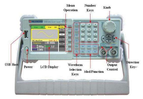
Figure 1-3 Front Panel of AWG Series
