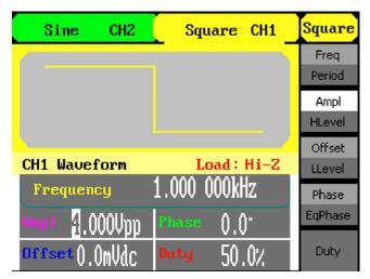
Figure 1-8 Square Signal Display Interface
