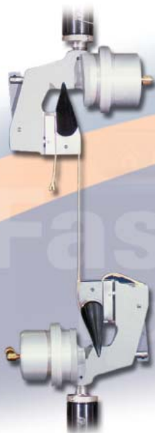
Automatic slack correction for textile specimens preserves correct strain values during testing.
