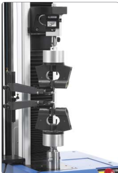
▲ ASTM D 412, rubber dogbone test
