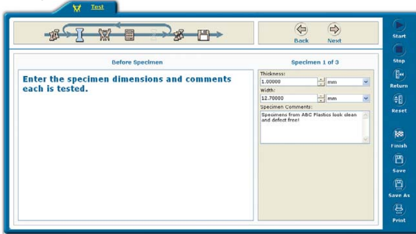
▲ 'Prompt' before the test specimen in testing mode
