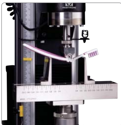
▲ Toothbrush flexural test
