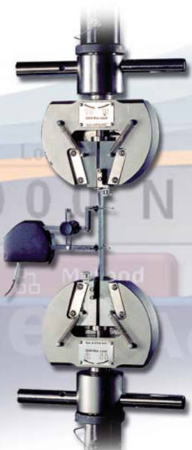
Driving to preload and balancing the extensometer preserves accurate results with no offset errors.
