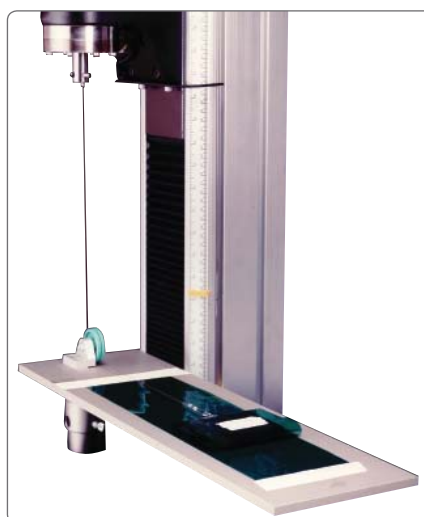
▲ ASTM D 1894 coefficient of friction testing
