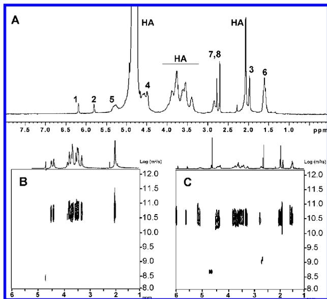
**Figure 1.** NMR characterization of the synthesized MeLAHA macromer.  $^1\text{H}$  NMR of the MeLAHA macromer with peaks matching labels of the final structure in Scheme 1 (A) and DOSY spectra of unmodified HA (B) and MeLAHA (C), indicating complete coupling.
