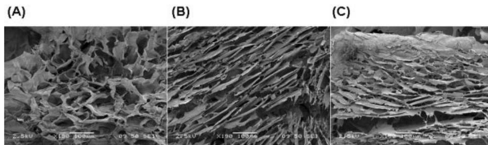
**Figure 1.** Scanning electron micrographs of (A) UV-cross-linked Az-chitosan, (B) noncross-linked Az-chitosan, and (C) chitosan. Scale bars = 100  $\mu\text{m}$ .
