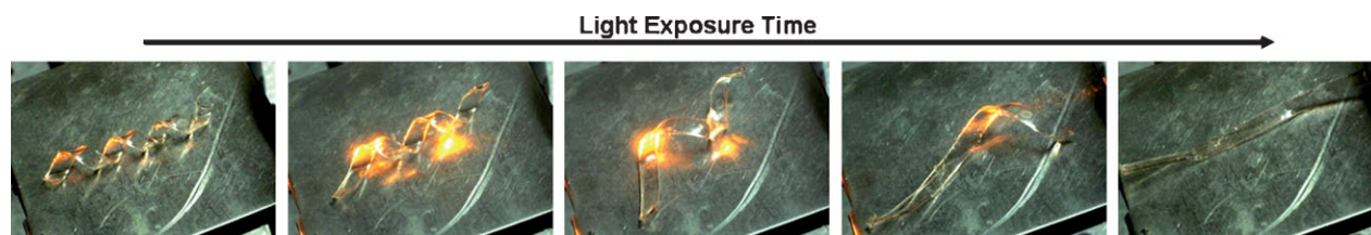
Figure 4. Images of shape transitions of polymers fabricated from 15:85 A6/tBA networks with nanorods (mid-concentration) after exposure to 0.3 W IR light. The complete transition took several minutes since the sample would change shape and move from the path of the light, yet shape changes were nearly instantaneous when the light was directed on the sample.
