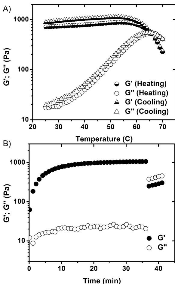
**Figure 1.** A) Dynamic oscillatory temperature sweep of PC10P gels (7 wt%, 10 mM phosphate buffer, pH 7.0) at a heating rate of  $2\text{ }^{\circ}\text{C min}^{-1}$ . B) Dynamic oscillatory time sweep of PC10P gels at  $25\text{ }^{\circ}\text{C}$  and an instantaneous temperature change to  $65\text{ }^{\circ}\text{C}$  at 35 min.
