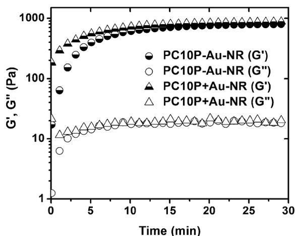
**Figure 2.** Oscillatory time-sweep measurements of PC10P gels with and without Au-NRs.
