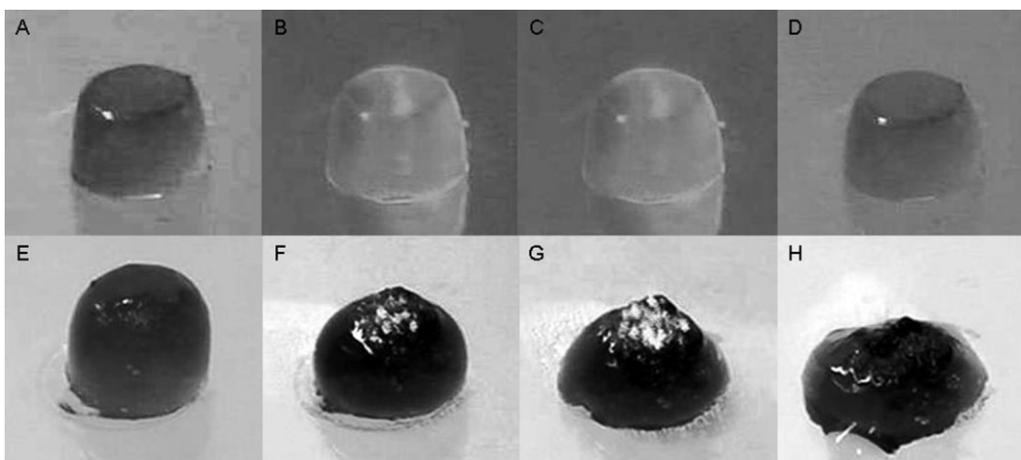
**Figure 3.** Snapshots of PC10P gels A–D) without and E–H) with Au-NR demonstrating melting of the gel only with Au-NRs: before NIR exposure (A, E), during NIR exposure (B, C, F, G), and after NIR exposure for 10 min (D, H).
