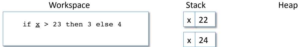
Figure 15.7: An example of how proper shadowing is implemented in the ASM. The value of the ready variable x will be found by searching the stack from most recent ( x maps to 24) to least recent ( x maps to 22).
