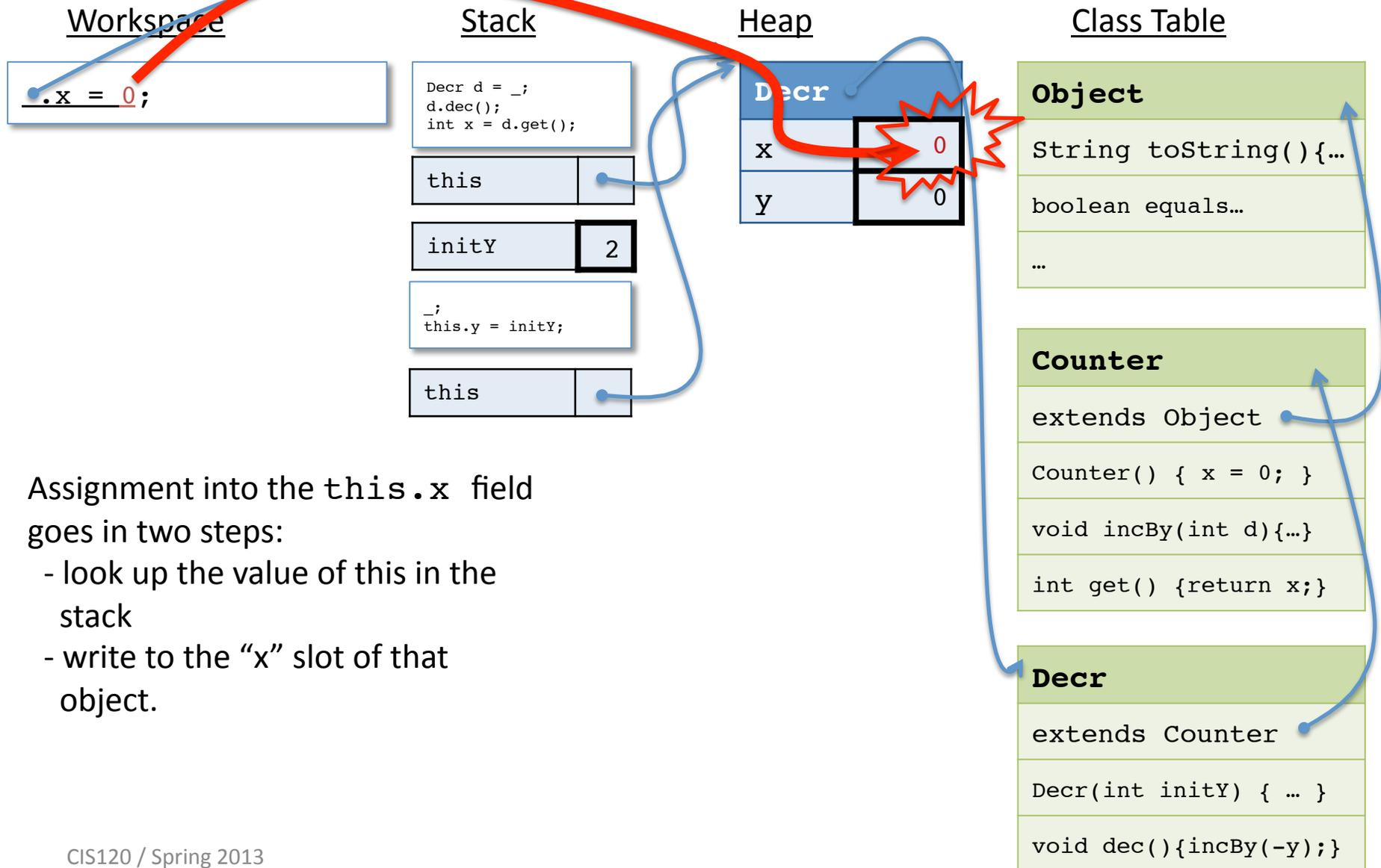
Assignment into the `this.x` field goes in two steps:
