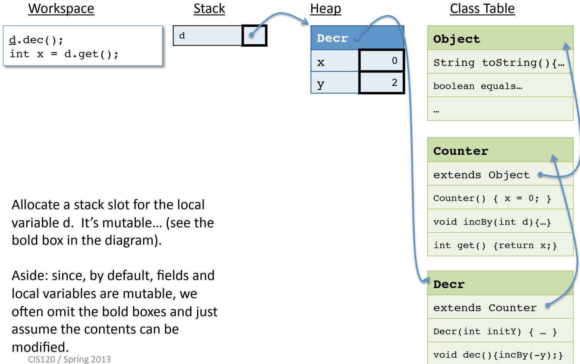
Allocate a stack slot for the local variable `d`. It's mutable... (see the bold box in the diagram).
