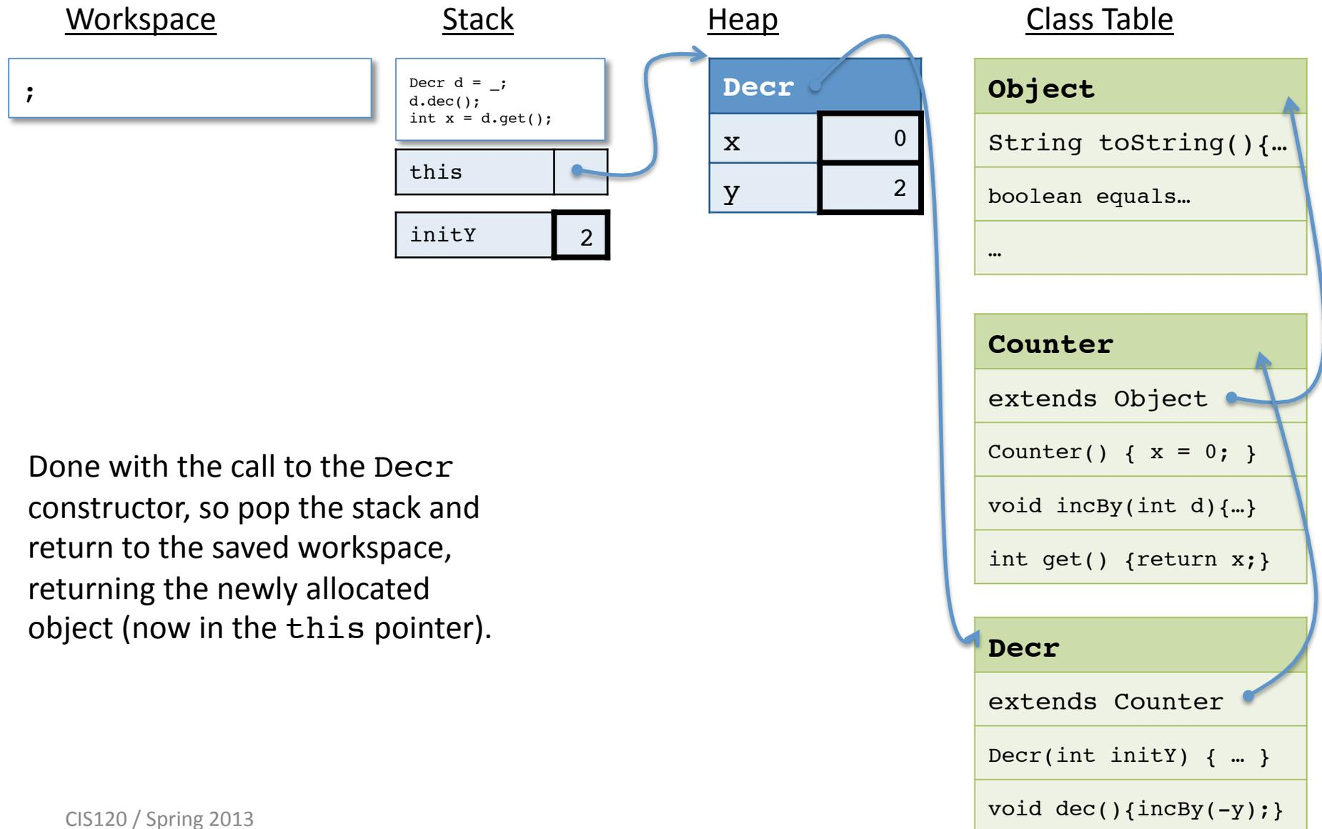
Done with the call to the `Decr` constructor, so pop the stack and return to the saved workspace, returning the newly allocated object (now in the `this` pointer).
