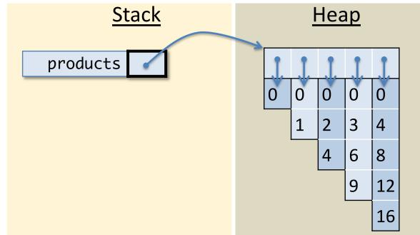
Note: This heap picture is simplified – it omits the class identifiers and length fields for all 6 of the arrays depicted. (Contrast with the array shown earlier.)
