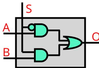
Input "S" selects A or B to attach to "O" output
