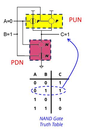
Note: parallel structure on top, series on bottom
