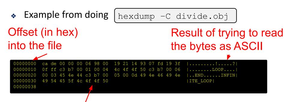
Contents of the file in hex, with spacing between each byte
