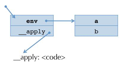
• Closure for function:  $\approx$  Instance of this class: class C { int a, b; int apply(x,y) { x + y + a + b } } D.V. apply а b \_apply: <code>
