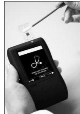
Prototype handheld genome sequencer
