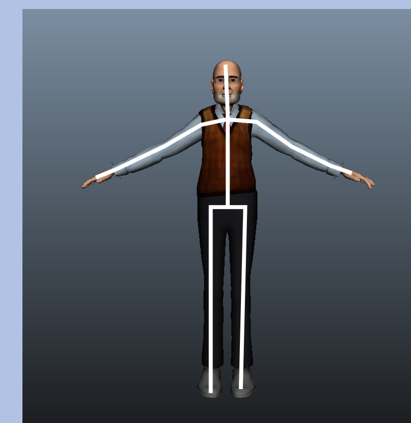
Compute the medial axis of the mesh by treating the faces as the loci of a 3D voronoi grid. The vertices of the voronoi diagram are the points of the medial axis. The grid cells are the places we compute the diagram.
