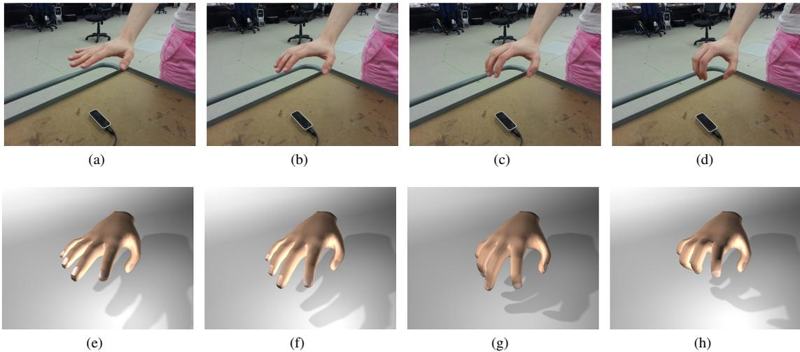
**Figure 1:** Top Left to Right: The Leap Motion controller tracks to palm and fingers above it. Bottom Left to Right: Our PAALM system estimates finger positions in real-time based on the Leap input. The bottom animation was created using a Maya plugin which communicates directly with the device to create keyframes for a hand model.
