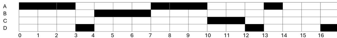
Note how there is a long time between the first time and second time task D ran; it simply became "runnable" after 3 time units of not running and was re-added to the queue until its turn.
