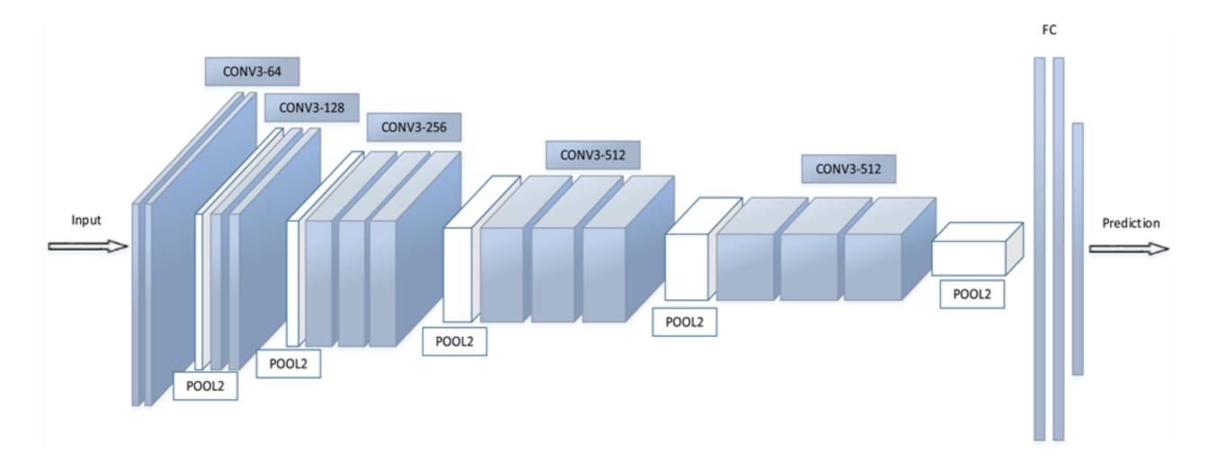
POOL2 : Max pooling done on windows of 2\*2 with **stride of 2**, so the height, width gets halved
