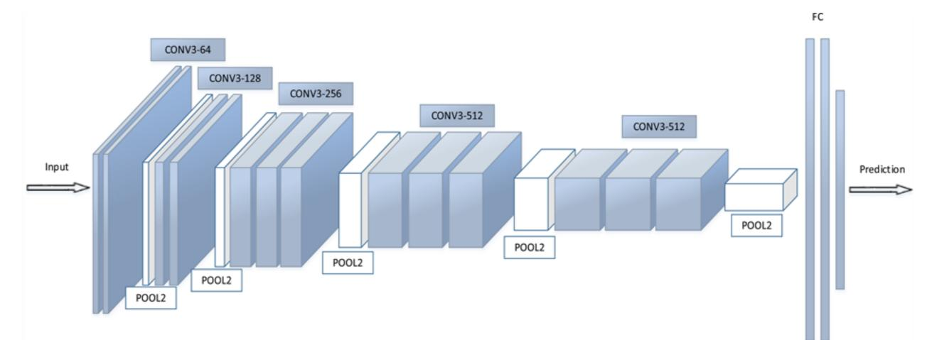
Thickness of each block corresponds to number of channels of the response / output. Height and width correspond to height and width of response / output.
