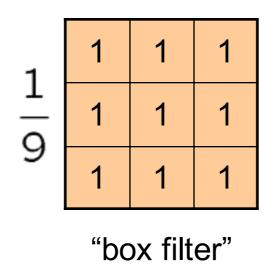
For each pixel **p**, place this matrix with the pixel **p** at the center. Perform point wise multiplication of matrix with pixel values, and average them. Make this the new value of pixel **p**.
