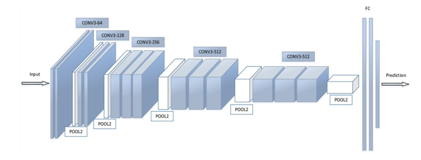
CONV 3-64 : convolutional layer with filters 3\*3\*(number of input channels), and 64 such filters are used. Each filter output also passed through **Relu activation**.
