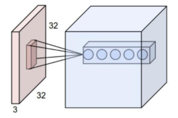
Each neuron in the convolutional layer is connected only to a local region in the input volume spatially, but to the full depth (i.e. all color channels). Questions ??
