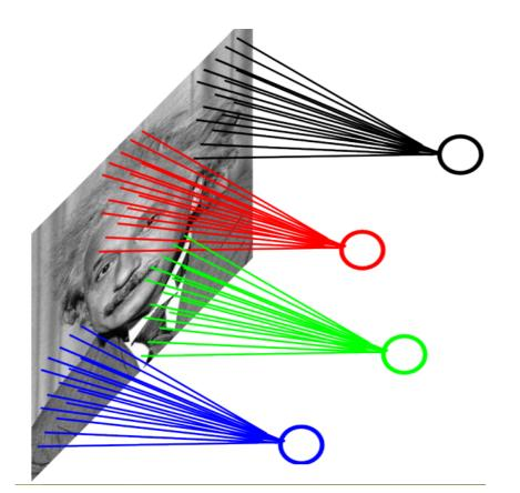
Each local region of the image is connected to a node in the next layer
