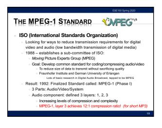
THE MPEG-1 STANDARD MPEG-1, (3) Layers for Audio Coding: Coding Required bitrate PCM CD Quality 1.4 Mbps 1:1 384 kbps Layer I 4:1 Complexity Layer II 8:1 192 kbps Layer III (MP3) 12:1 128 kbps Why is PCM CD Quality 1.4 Mbps? Recall: 1 sec. of music: 44,100 x 16bits = 705,600 bits Don't forget stereo (R/L): 2 x 706,600 = 1,413,200 (1.4Mbs) Defines bandwidth requirements of network Notice: 128 kbps was just about double modem speed in 1992 Enables transmission of audio (MP3) via modem!
