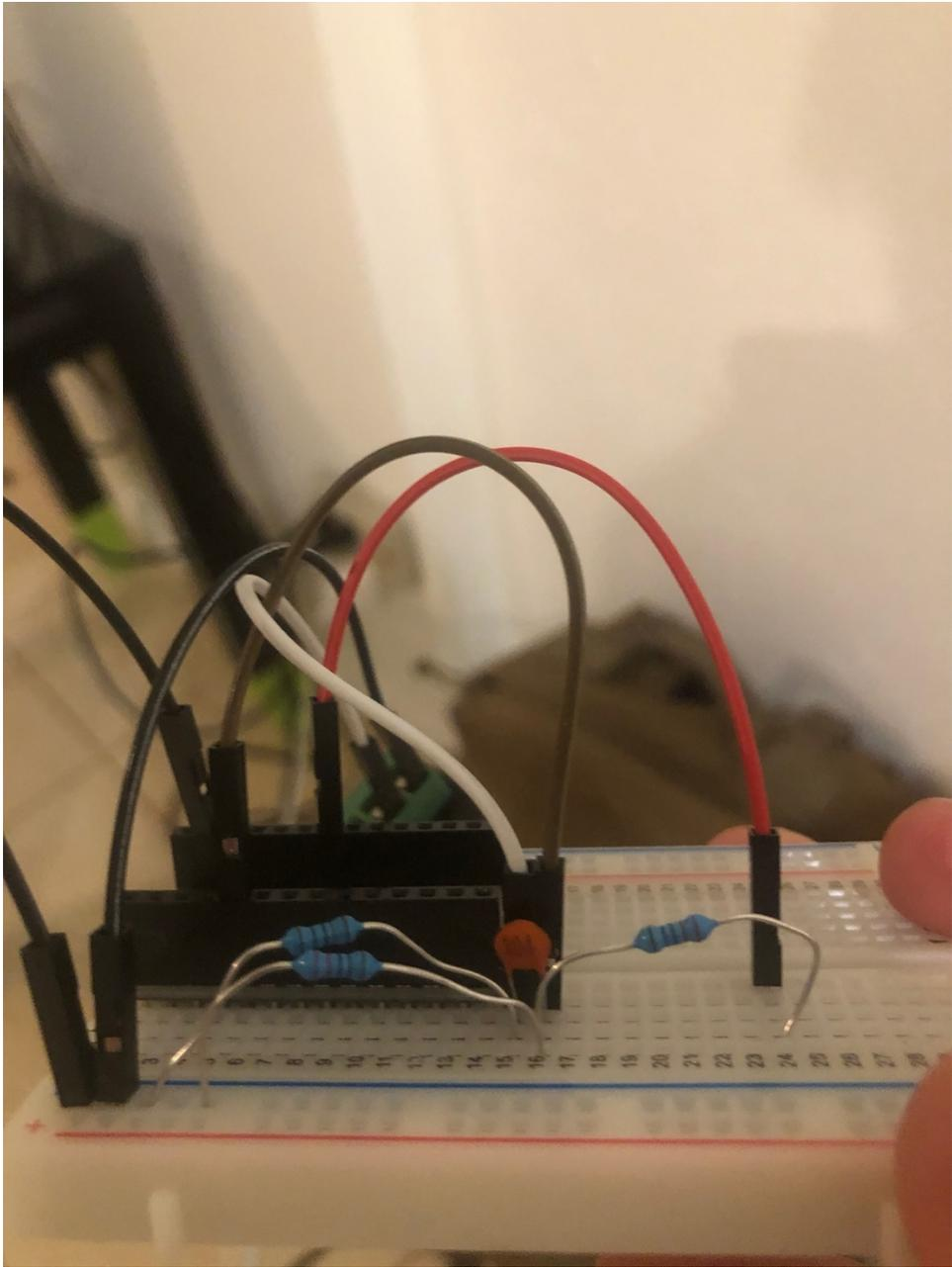
Finally, connect the audio input wire into the same row of the capacitor as the 1kOhm resistor. Connect the other side of the last 10K Ohm resistor to the USB pin of the Itsy-Bitsy, and connect the other side of the capacitor to pin A0. The final product should look like this:
