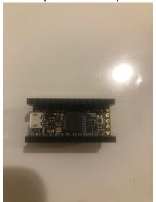
You should notice *female* wire connectors in addition to the USB type-c connector. The wire connectors will allow us to connect different components to
