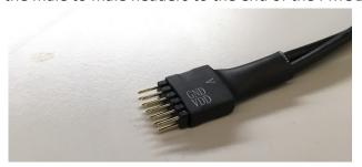
ii. Connect the Pmod buttons to the end of the Pmod extension cable that has 6 holes and is labeled A, and the Pmod switches to the other end. The buttons and switches should look as follows:
