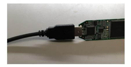
v. Lastly, connect the FPGA to the Windows computer (the larger of the two Dell machines) at your lab station. Plug into the leftmost USB port on the main computer box.
